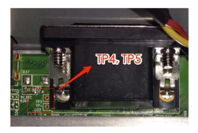
STEP3: Disconnect the DVR power. Then, make the chip resistor short-circuited with a conductive object (such as forceps), and re-connect the power. Remove the conductive object when you hear a short beep sound, and wait till the DVR reboots.
