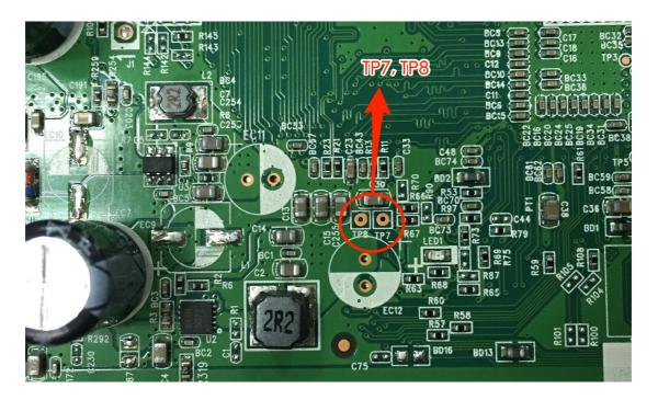
STEP3: Disconnect the DVR power. Then, make the chip resistor short-circuited with a conductive object (such as forceps), and re-connect the power. Remove the conductive object when you hear a short beep sound, and wait till the DVR reboots.
